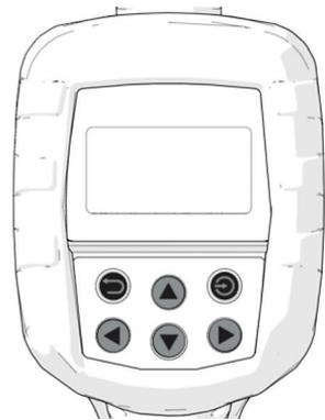
The gun automatically switches off after 30 seconds of inactivity to save energy. To turn the display back on, press any of the UP/DOWN keys. Once the display is activated, the name of the equipment is briefly displayed along with the
