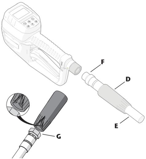
To connect the hose, hold the hose end (F) stationary while turning the swivel end (G) until the desired tightness is achieved.
